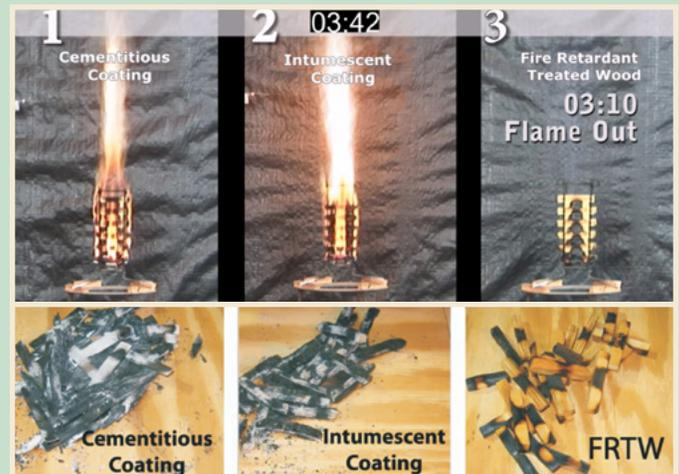
As the ASTM E160 test demonstrates, FRTW self-extinguishes when the burner is removed at 3 minutes. Coated wood does not self-extinguish and continues to burn until it is completely reduced to nothing but ash and coating residue.
