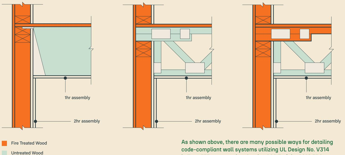
As shown above, there are many possible ways for detailing code-compliant wall systems utilizing UL Design No. V314 in Type III construction. Section 602.3 of the 2018 IBC was clarified to show that FRTW plywood sheathing complying with Section 2303.2 is allowed in the exterior bearing walls of Type III construction.
